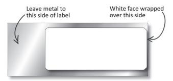
Smallest recommended bending diameter of the Confidex Silverline Blade $^{\text{TM}}$  is 100mm. For optimal performance please bend the label in the orientation shown below.
